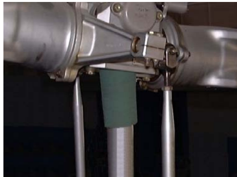
Figure 2. OH-58A/C Mast Wedge Assembly
